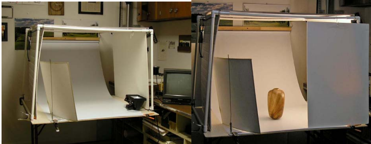
Photo 1. Frame is 1/2" PVC pipe, sides measure 34"x34" and top is 44" wide. Backdrop is white vinyl roll-up window shade. I often plug camera video into this monitor for enhanced view of camera image.
